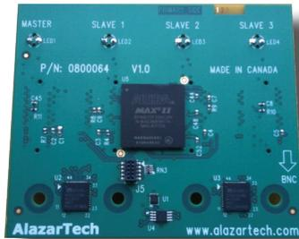
SyncBoard-9440 is a mezzanine board that connects to the Master/Slave connector along the top edge of the ATS9440 and sits parallel to the motherboard. For additional robustness, users can secure the SyncBoard-9440 to a bracket mounted on each of the ATS9440 boards.
