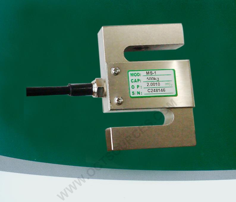
S type load cell, tension and compression Good output symmetry, compact structure, simple to install, full range of capacities Suitable for electromechanical scale, crane scale, hopper scale and various special scales
