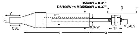
CL (Cable length). - See specification. CSL (Cable sleeve length). - See specification.
