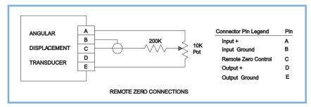
Unless operating in a noise free environment, the lead to pin C must be shielded, as shown. The existing zero adjust potentiometer in the Angular Displacement Transducer must be rotated fully clockwise before the remote zero control can function correctly. This remote function is useful in applications where it is inconvenient to access the adjustment screw on the transducer housing.
